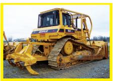
2005 CAT D6RXL SNAAX00929 Cat diesel engine. equipped with EROPS, SU blade, 3rd valve hydraulics, rear ripper, long track frame.
