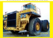
**KOMATSU 630E** SNGF32002AFE46M Detroit diesel engine, equipped with Cab, Red Dot air, 190 ton capacity dump body, 33.00-51 tires.
