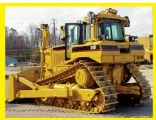
CAT D8R SN7XM4071 Cat diesel engine, equipped with EROPS, air, 8SU blade with tilt, New Cat 24in. undercarriage.
