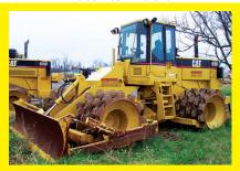
2004 CAT 815F SN0BL00913 Cat diesel engine, equipped with EROPS, air, straight blade with tilt, (4) padsfoot drums.
